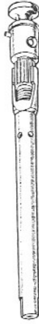
The slow-running device of the Zenith Carburettor, showing the screw adjustment and locking arrangement. In the carburettor itself it is placed vertically.
