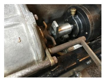
The little control rod ends are a Vauxhall trademark, and it would be lazy to use a proprietary substitute:
