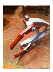
I splattered on a ¼" strap top and bottom:
