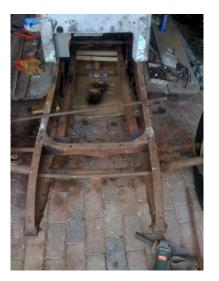
New cross tube and brackets cast and machined:
